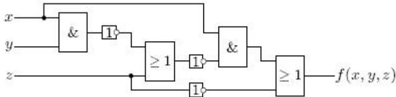
Write down the function computed by this circuit. Find the table of values, and write the function in both conjunctive and disjunctive normal form. Furthermore, make the transformation from the original to the disjunctive normal form using the rules in table 7.3. Draw a circuit that computes the function using the normal form of your choice.
